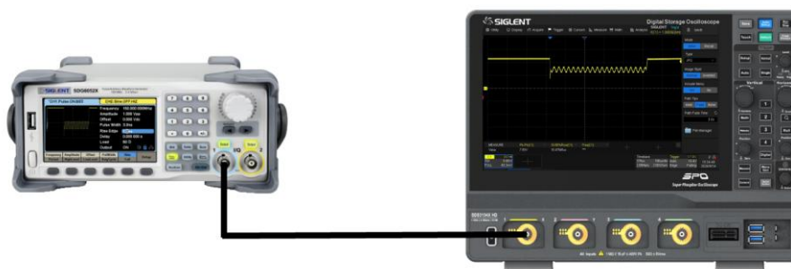
Figure 4: setup to adjust the output signal
