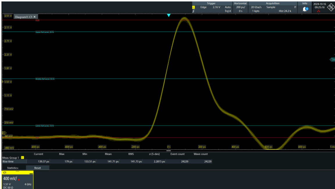
Picture 7: output pulse, 20 MHz base frequency, 50Ω termination
