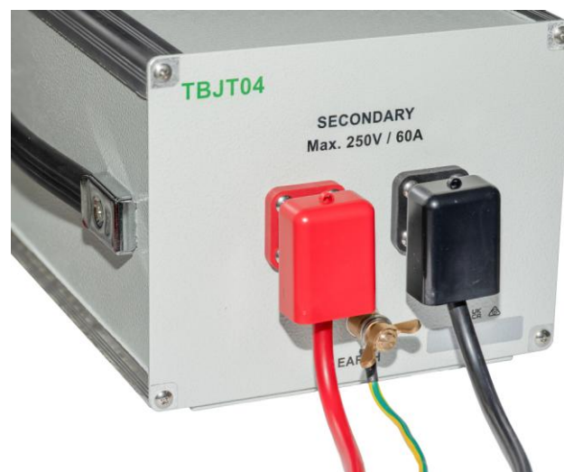
Picture 2: protection covers attached to the secondary terminals
