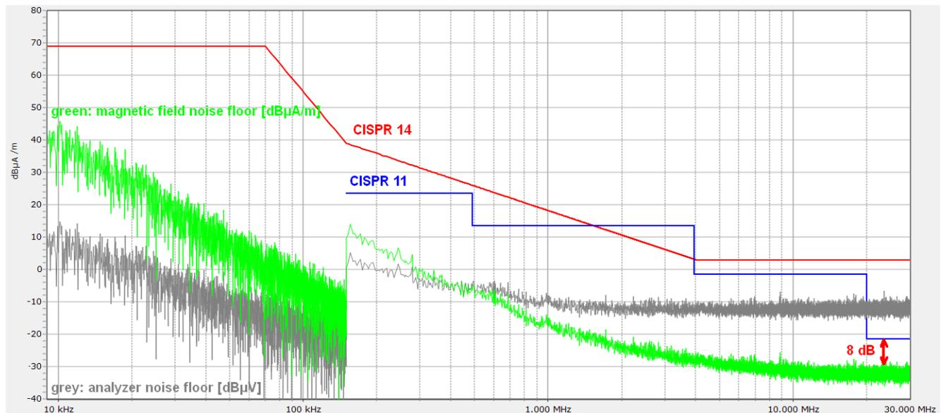
The above screenshot shows the magnetic field noise floor of a set up consisting of a low-cost spectrum analyzer and the TBMA6-P loop antenna.
