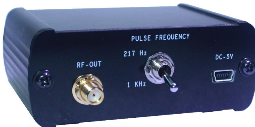
Picture 1 – TBMDA1 modulated wideband driver amplifier front view
