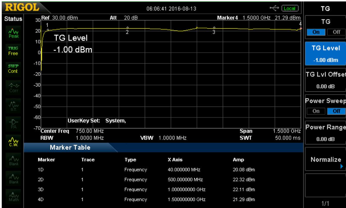
Picture 7 – output power of the TBMDA1, CW, driven by the DSA815 tracking generator set to -3dBm
