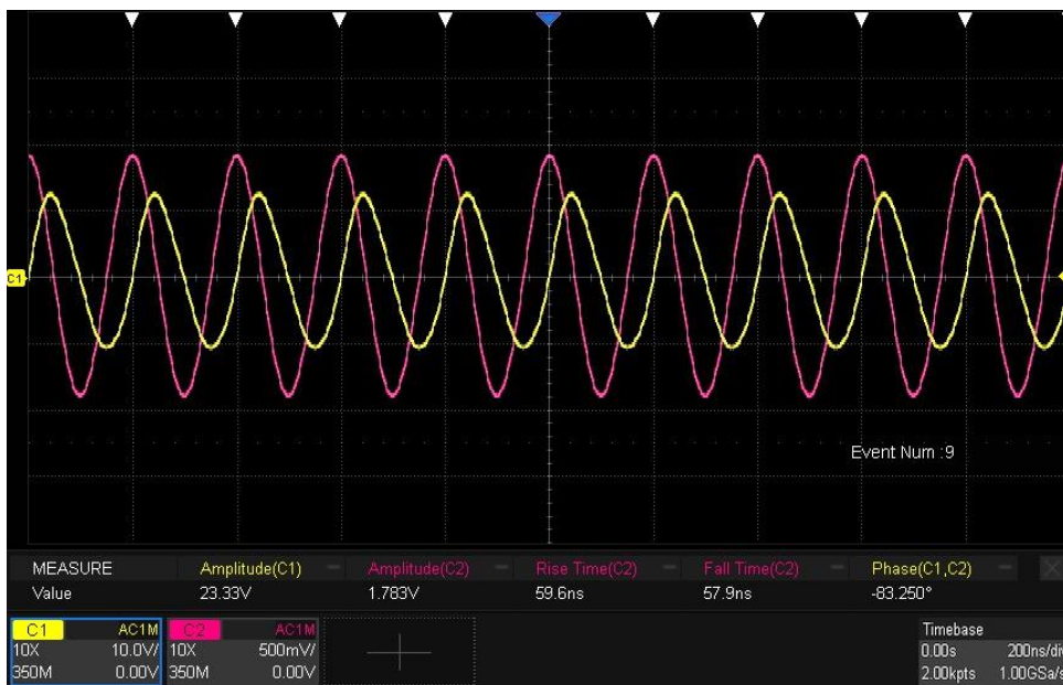
Figure 18: Output loaded with 0.5 Ohm wire wound resistor, 5 MHz; 23 Vpp, 1.8 App
