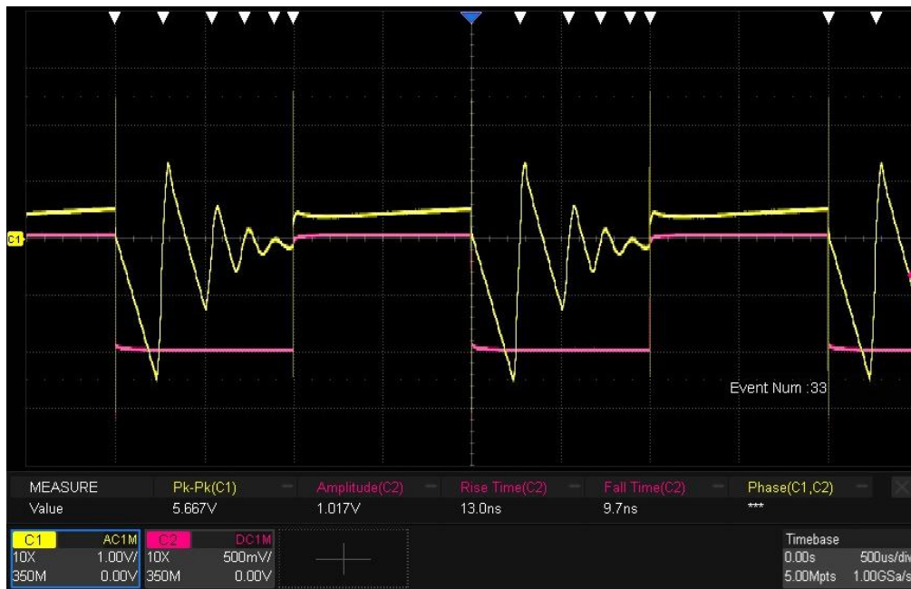
Figure 15: load transient measurement
