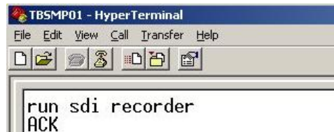
Figure 8 –TBS03 Transfer mode initialization using Windows Hyper Terminal
