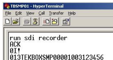
Figure 9 –TBSMP02, sensor response to ID command 0!!
