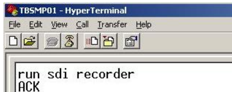
Figure 8 –TBS03 Transfer mode initialization using Windows Hyper Terminal
